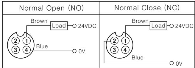
※ ②, ③ of NO Type and ③, ④ of NC Type are N · C (Not Connected) terminals.
