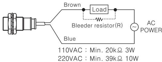
If the load current is under 5mA, please make sure the residual voltage is less than the return voltage of the load by connecting a bleeder resistor in parallel with the load as shown in the diagram.
