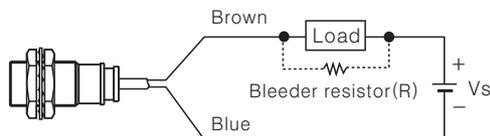
Please make the current on proximity sensor smaller than the return current of load by connecting a bleeder resistor in parallel.
