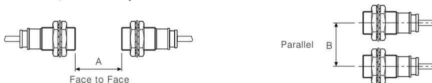
When sensors are mounted on metallic panel, you must prevent the sensors from being affected by any metallic object except target. Therefore, be sure to provide a minimum distance as below chart.
